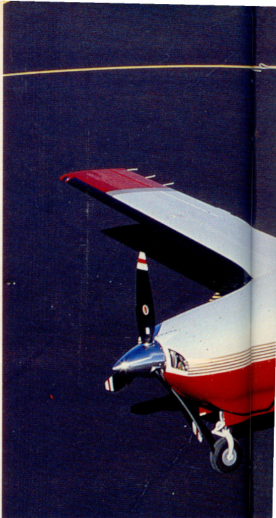
Among the most significant external changes to the new Mirage are the three-blade propeller and recontoured exhaust tunnels (above). Inside, the annunciator panel (left) and systems control panel are new.
